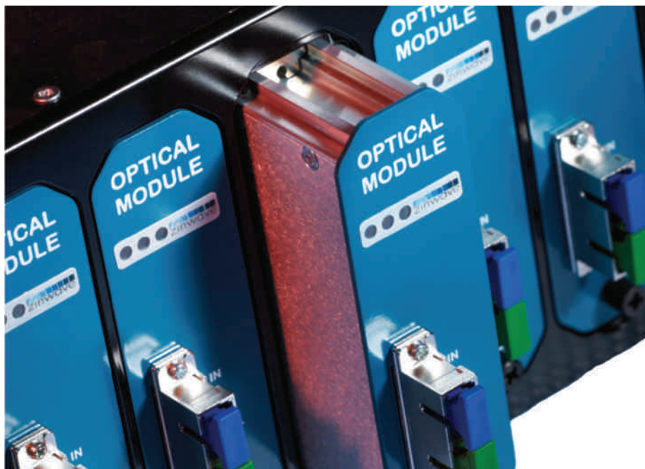
Zinwave’s technology relies on uncooled laser diodes to achieve cost-effective operation.
